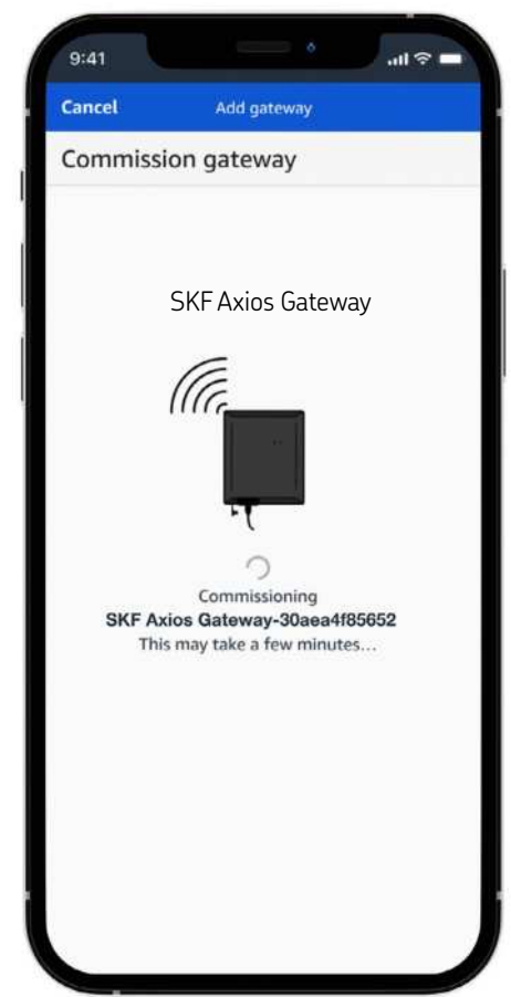
4 Once commissioning is complete, you can verify the gateway is online by the solid orange light.
